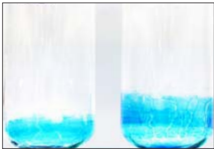
Fig.5: Grease sticking to the glass wall obtained from a 170 RPM (left) and a 300 RPM (right) concentration.
