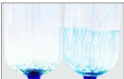
Fig.6: Oil sticking to the glass wall after a concentration with (left) and without (right) Flushback Module.
