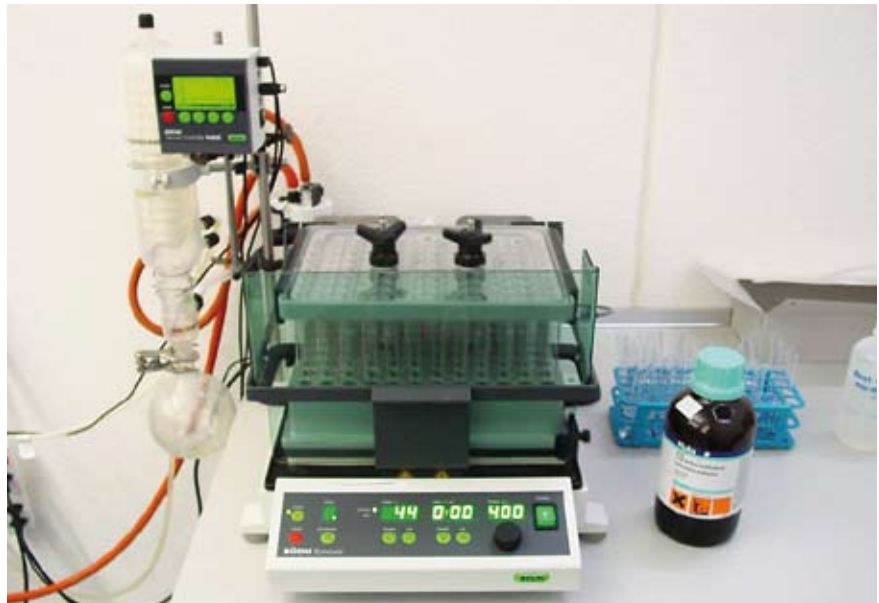
Figure 3: Laboratory equipment used for parallel evaporation under vacuum according to the modified BGIA method. The Syncore® Polyvap with a 96 position rack was used to heat the samples to 60 °C and to generate a vigorous vortex at 400 rpm. In order to avoid cross-contamination due to condensation, the vacuum cover was heated to 45 °C. A vacuum was generated using the V-500 vacuum pump and controlled with a pressure profile programmed with the V-805 vacuum controller (see Figure 2).
