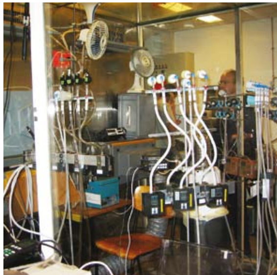
Figure 4: Round robin inter-laboratory sampling exercise in an experimental chamber of 10 m 3 . Oil mist was generated with light, medium and heavy mineral oils based MWF (Somentor 29, Blaser VP 1006 or Blasomil 22 and Blaser 220 respectively) in a home-made glass nebulizer. The generated range of oil mist can be regulated in the range of 0.1 to > 20 mg/m 3 and can be held constant at least for 6 hours within a deviation standard of < 5%. The spatial uniformity of the aerosol inside the test chamber was in the range of 2 - 3% reported by 5 point test.
