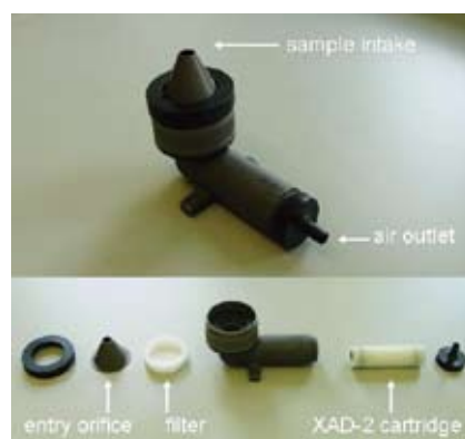
Figure 1: GSP sampler with a Ø 37 mm filter and 3 g XAD-2 cartridge used for the BGIA-modified procedure.
